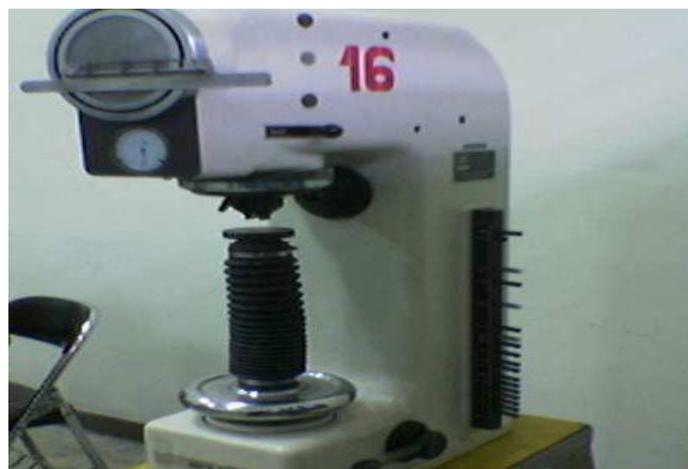
**Gambar 6.** Mesin Kekerasan Universal
